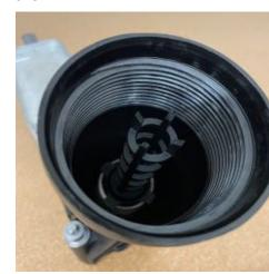
**Step 6:** Install body O-ring seal and lubricate with engine oil.
