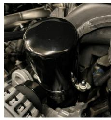
**Servicing instructions at Oil Change:** Prior to oil filter removal and draining engine oil from the oil pan, apply minimum 30 PSI to the Schrader valve
