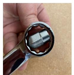
**Step 8:** Lock the adapter in place, by tightening the socket head cap screw with a 5/32 hex wrench.
