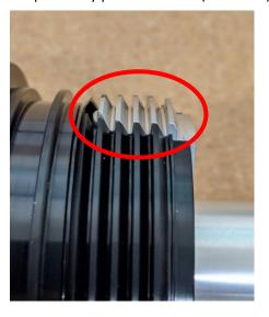
**Step 3:** Install the Adapter until it bottoms out, then back it out less than 180 degrees to expose an NPT port to be utilized for the Schrader valve. Note the orientation (the opposite one will be plugged with the included hex plug) and remove adapter.
