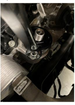
**Step 7:** Install schrader valve.
