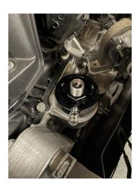
**Step 8:** Install appropriate size oil filter that contains M22x1.5 threads.
