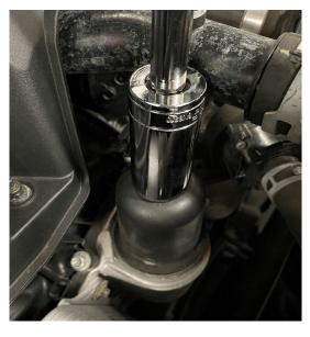
**Step 3:** Install adapter without body and tip O-rings.
