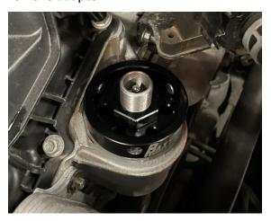
**Step 2:** Lubricate internal O-ring on docking collar.
