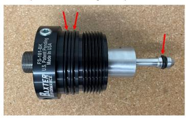
**Step 6:** Lubricate threads with oil and install 90° fitting (if using) with 15/16" 12-point wrench.
