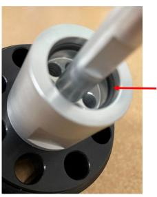
**Step 4:** Lubricate hex plugs with oil and install in two ports not utilized using a 3/16 hex wrench.
