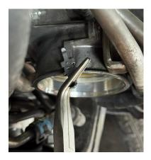
5. Install body O-ring and lubricate with engine oil.
