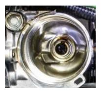
4. Apply sealant tape (not included) to hex plugs and install in unused ports using 3/16" hex wrench.
