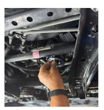
8. Install spin-on oil filter that contains ¾-16 threads, run engine and check for leaks.
