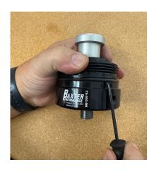
3. Test fit - Using 1" deep socket, install adapter until fully seated. Determine which port will be utilized for the Schrader valve. Remove adapter.
