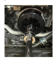
7. Install 90-degree fitting with sealant tape (if using) and Schrader valve.
