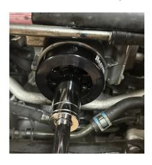
6. Install adapter using 1" deep socket, torque to 40 ft.lbs.
