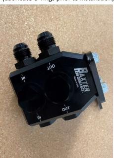
**Step 5:** Install remote mount assembly using 3 ea. 8mm bolts.
