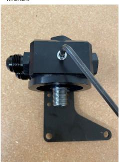
**Step 5:** Install appropriate size oil filter that contains ¾-16 threads.
