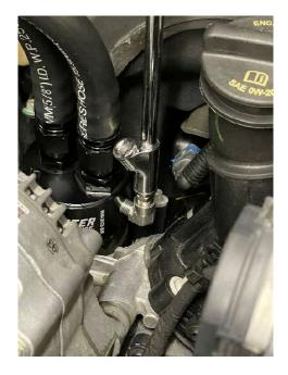
Note #1 Teflon sealing tape may be used instead of oil on plug, 90 degree fitting or Schrader valve. Be certain to apply tape to threads only and not over the end, this will avoid possible contamination of oil system.
