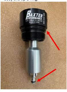
installed using a 15/16" 12 point closed end wrench.
