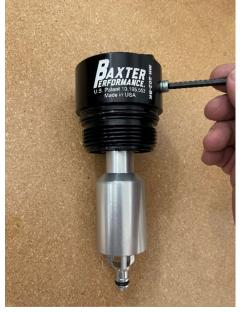
Step 2: Test fit for alignment and clearance prior to O-ring installation.
