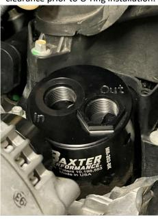
Step 4: Install adapter with 1 1/8" socket. Helpful Hint: 90-degree fitting can be Apply oil to 90 degree fitting and/or Schrader valve and install. See Note #2
