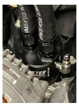
Servicing instructions at Oil Change: Prior to draining engine oil from oil pan, and oil filter removal, apply 30 PSI minimum/60 PSI max to the Schrader valve, this will evacuate the oil retained in remote oil filter and external oil cooler if installed. Then, remove oil filter and replace.
