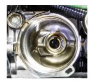
Remove cartridge filter cap assembly.
